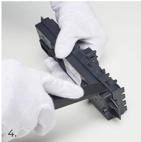
4. Insert the wedge into the side gap between the top and bottom parts of the assembly at the latch location, pushing it in up to the edge of the latch.
