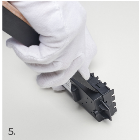
5. Move the wedge upwards to release the latch.
