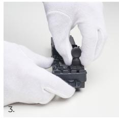
Gently press down on the switch from above and snap its outer side protrusion into the assembly.
