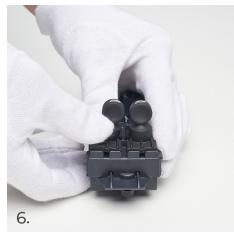
Gently press down on both the front and rear parts of the switch base simultaneously and snap its outer side protrusion into the device.
