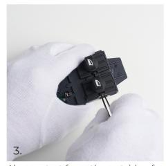
Always start from the outside of the switch. Start from the top and place the tweezers in the area shown in the previous image.
