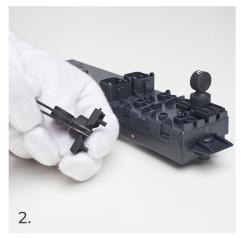
This is where you need to place the top of tweezers to prevent switch damage.
